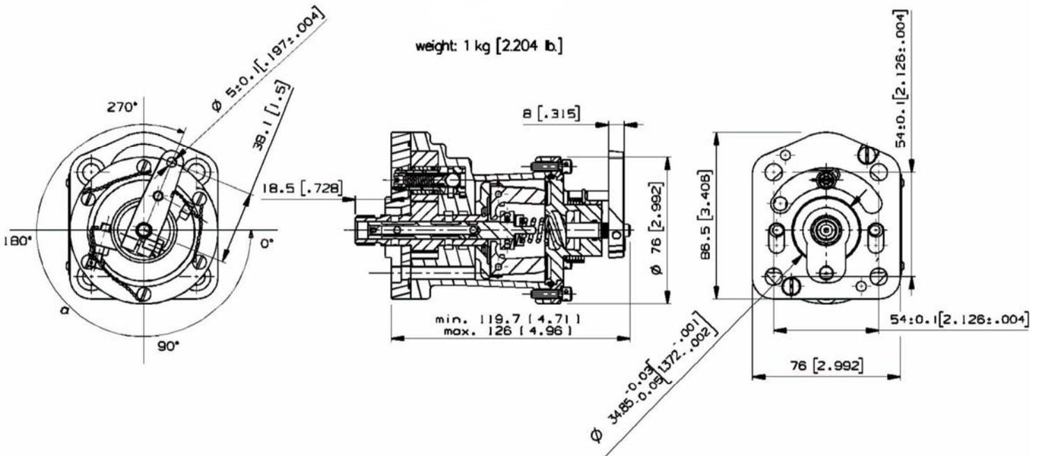
Note: Operating lever as shown is set at 290° for counter-clockwise rotation
